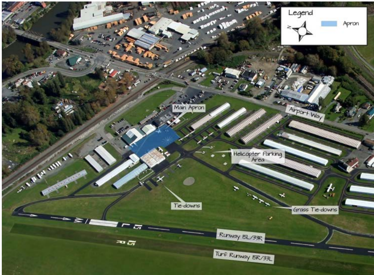
FIGURE 4-4 – AIRCRAFT PARKING APRON/TIE-DOWNS
